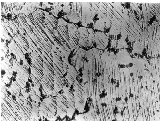
Fig. 10. Deformed molybdenum weld deposit (500 \times ).
